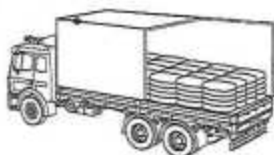
It is not necessary to attach the load if it is loaded in an enclosed or roofed vehicle and is light enough so that it does not change the vehicle's centre of mass in the event of spreading.
