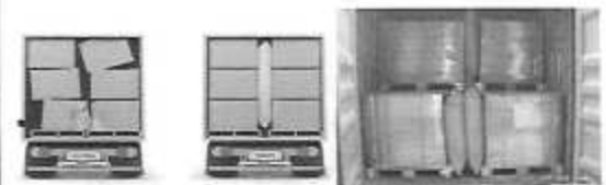
Securing the load with inflatable devices.
