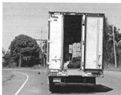
The load is not secured at the rear.
