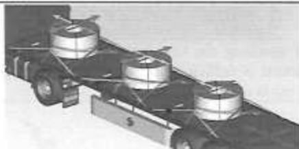
Vertical attachment of the heavy rollers, the brown belt restricts the yellow and blue belts from sliding down.
