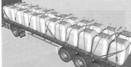
IBC (big bags) fastening. A spring clip is used at the ends and in the middle.
