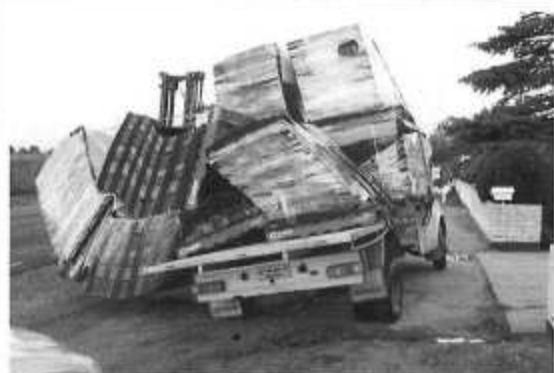
The lashing belts are insufficiently tensioned.
