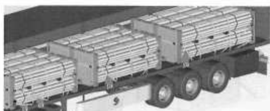
Fastening of short rods or pipes using a pallet.
