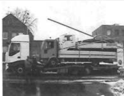
Incorrect loading - centre of gravity too high, vehicles are unstable due to the spring chassis.
