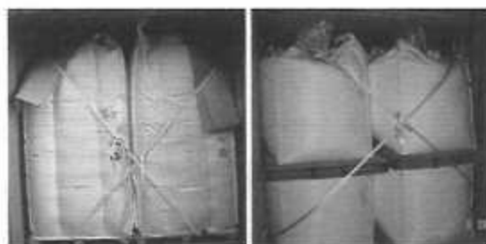
Closed large bags can be secured in this way.
