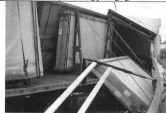
Mounting wedges are missing or insufficiently secured.
