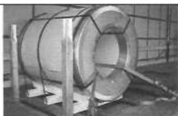
Cross-mounting of the roller with additional supports.
