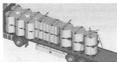
Fastening drums and lightweight bales with packs.
