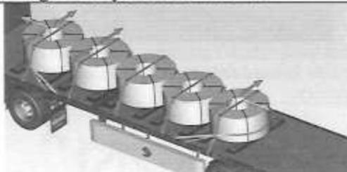
Vertical roller mounting, brown belt restricts the yellow and green belts from sliding down.
