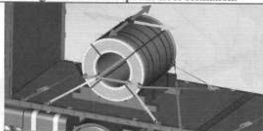
The mounting of the roller is transverse. The green and red attachment straps are held in place by the yellow straps.
