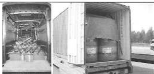
Loads can be secured with mesh or cover.
