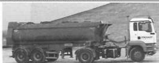
It is not necessary to attach the load if it is transported in bulk and cannot crumble when travelling over bumps in the road.
